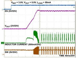
FIGURE 10. START-UP AFTER ENABLE (I<sub>LOAD</sub> = 50mA)
