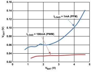
FIGURE 6. LINE REGULATION,  $V_{OUT} = 5V$
