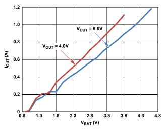
FIGURE 5. MAXIMUM OUTPUT CURRENT vs INPUT VOLTAGE
