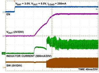
FIGURE 9. START-UP AFTER ENABLE (I<sub>LOAD</sub> = 250mA)
