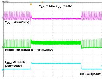
FIGURE 11. LOAD TRANSIENT RESPONSE (100mA TO 500mA)
